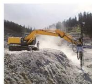
Attachment drill with hydraulic rock drill
