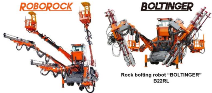
Fully automatic drill jumbo "ROBOROCK" J32RX-Hi
