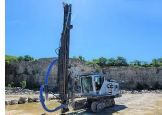
Hydraulic crawler drills
