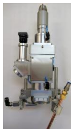
Laser head equipped with DOEs
