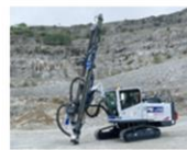
Hydraulic crawler drill with a semi-automatic drilling function
