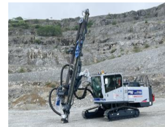
Hydraulic crawler drill with a semi-automatic drilling function
