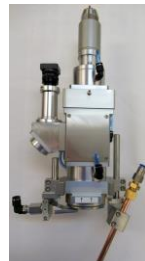
Laser head equipped with DOEs
