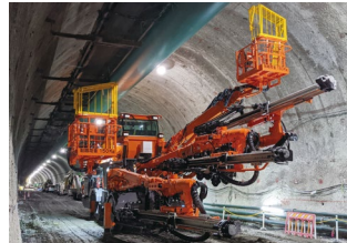
Fully automatic drill jumbo
