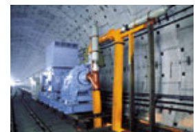
Slurry pump for tunnel shield construction
