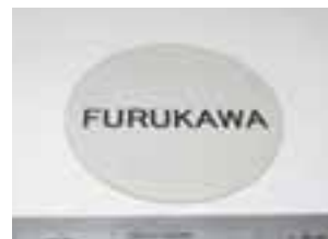
A two-inch diameter gallium nitride substrate
