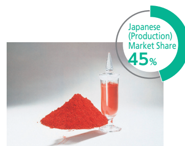
Cuprous oxide is a red powdery substance used to prevent corrosion on the underside of marine vessels.
