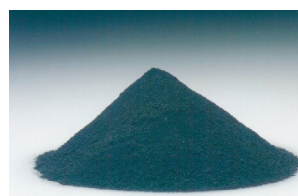
Cupric oxide used for copper plating
