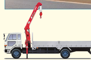
Truck-mounted UNIC crane
