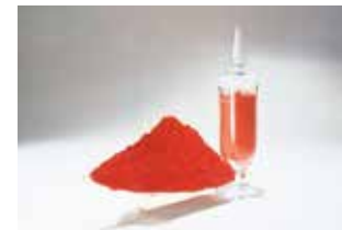
Cuprous oxide is a red powdery substance used to prevent biofouling on the underside of marine vessels.
