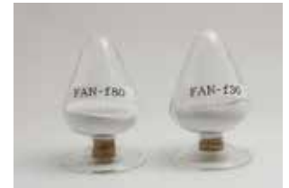
Owing to its excellent thermal conductivity, thermal radiation, and electrical insulation properties, aluminum nitride is a basic material used in semiconductor device fabrication components and substrates.
