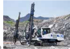
Hydraulic crawler drills
