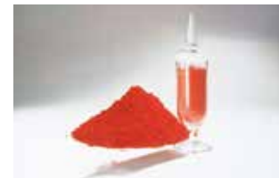
Cuprous oxide is a red powdery substance used to prevent biofouling on the underside of marine vessels.
