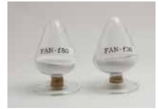
Owing to its excellent thermal conductivity, thermal radiation, and electrical insulation properties, aluminum nitride is a basic material used in semiconductor device fabrication components and substrates.
