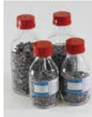
High-purity metallic arsenic—high-purity gallium arsenide semiconductor materials used in mobile phones and other electronic devices, red laser diodes, and LEDs
