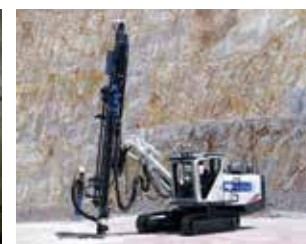
Hydraulic crawler drills
