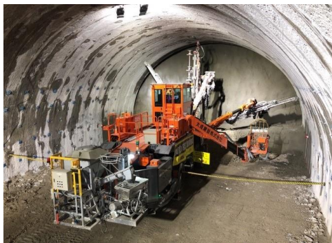
The BOLTINGER, a rock bolting machine equipped with a six-meter joint bolt placing device. (Jointly developed with Taisei Corporation.)
