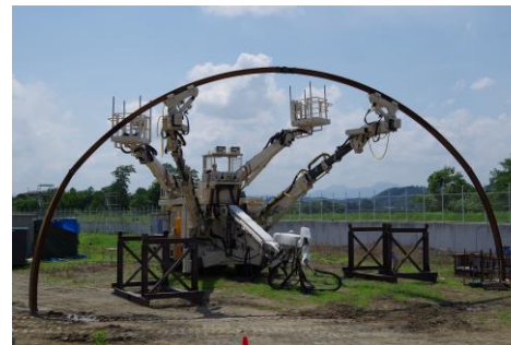
Tunnel drill jumbo using remote technology. (Jointly developed with HAZAMA ANDO CORPORATION and MAC.)
