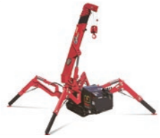
Mini crawler cranes Outside Japan, these cranes are used on construction sites for skyscrapers and the like.
