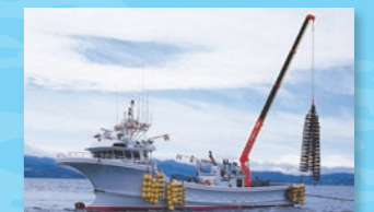
Ocean cranes These machines are used in oyster farming and unloading catches from vessels.
