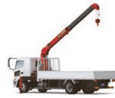
UNIC cranes These truck-mounted cranes are used on construction sites and the like.
