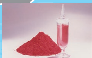
Cuprous oxide This eco-friendly substance is used to coat the undersides of marine vessels.
