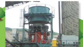
Crushers These machines crush rocks into smaller pieces at quarry.
