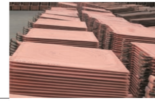
Electrolytic copper This substance is used in the wires, copper pipes, and other components of household appliances, communication devices, and automobiles.
