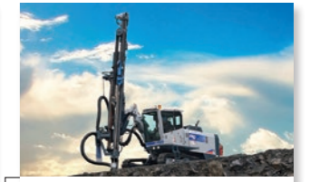
Hydraulic crawler drills These machines drill holes for blasting at stone-crushing plants and limestone mines.
