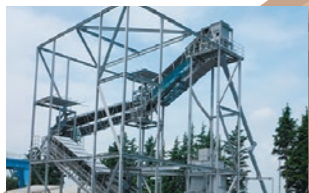
Enclosed suspended conveyors These conveyors are used to close off and vertically transport materials.
