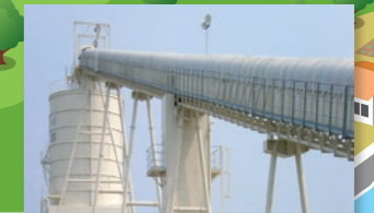
Belt conveyors This equipment transports massive amounts of earth and sand, ore, coal, and other raw materials.
