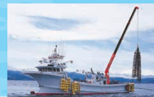
Ocean cranes These machines are used in oyster farming and unloading catches from vessels.
