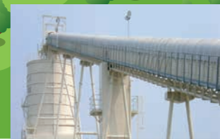
Belt conveyors This equipment transports massive amounts of earth and sand, ore, coal, and other raw materials.
