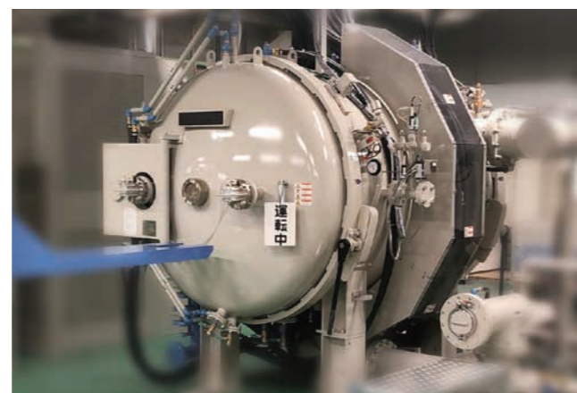
A furnace for manufacturing aluminum nitride ceramics
