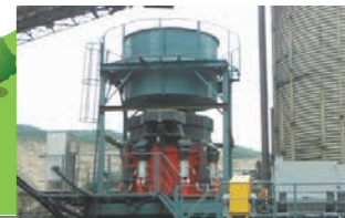
Crushers These machines crush rocks into smaller pieces at quarry.
