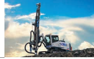
Hydraulic crawler drills These machines drill holes for blasting at stone-crushing plants and limestone mines.
