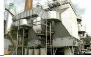
Electrostatic precipitators This equipment prevents air pollution from plants and other facilities.
