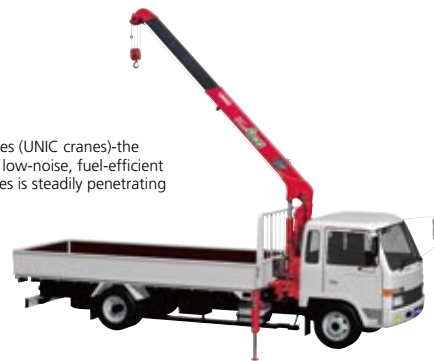
Vehicle carriers (UNIC carriers)-the UNIC carriers lineup of high-value-added products includes truck-mounted cranes that can operate on a platform with a 1° angle and two-vehicle carriers.
