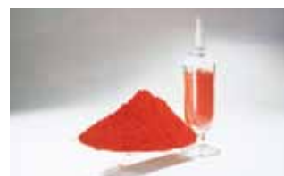
Cuprous oxide is used as an antifouling agent in paints applied to the bottoms of ships.
