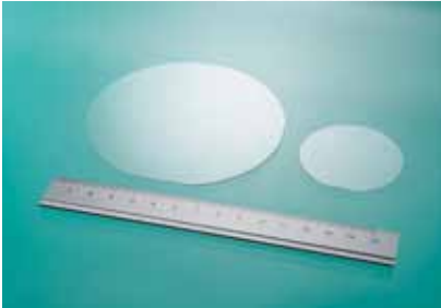
Two-inch GaN substrate and the recently developed four-inch GaN substrate
