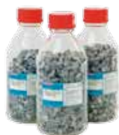
High-purity metallic arsenic—high-purity gallium arsenate semiconductor materials used in mobile phones and other electronic devices, red laser diodes, and LEDs
