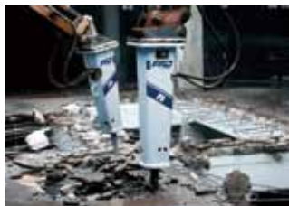
Hydraulic breakers, which are attached to hydraulic shovels, are used for excavating rock and breaking concrete.
