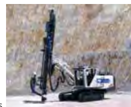
Hydraulic crawler drills
